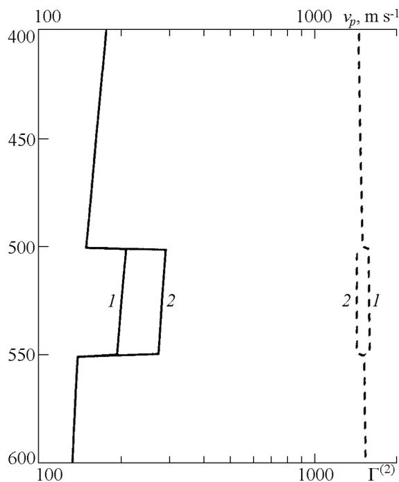
**Figure 4.** Velocity of longitudinal waves (dashed line) and parameter of quadratic nonlinearity (solid line) versus depth in the presence of fluid-impermeable dome and at partial unloading of intergranular contacts due to pressure in pore fluid; 1, gas content  $\beta = 0$ , and 2,  $\beta = 0.01$ .
