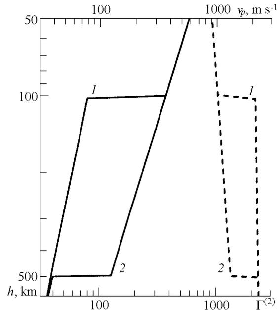
**Figure 2.** Velocity of longitudinal waves  $v_p$  and parameter of quadratic nonlinearity  $\Gamma^{(2)}$  versus depth  $h$ ; 1, for top of a fluid-bearing layer,  $H_0 = 100$  m and 2,  $H_0 = 500$  m. Dashed line shows velocity of longitudinal waves and solid line shows the parameter of quadratic nonlinearity.
