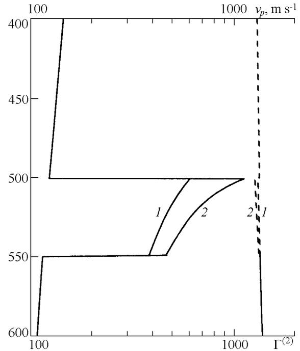
**Figure 3.** Velocity of longitudinal waves  $v_p$  and parameter of quadratic nonlinearity  $\Gamma^{(2)}$  versus depth  $h$  in the presence of fluid-impermeable dome. Unloading of intergranular contacts by pore fluid is close to maximal. Dashed line represents velocity of longitudinal waves, and solid line represents the parameter of nonlinearity; 1,  $k = 0.95$ ; 2,  $k = 0.985$ .
