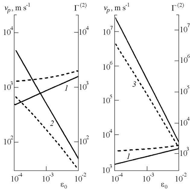
**Figure 1.** Velocity of longitudinal waves and nonlinearity parameters versus initial strain  $\varepsilon_0$ ; 1, velocity of longitudinal waves  $v_p$ ; 2, parameter of quadratic nonlinearity  $\Gamma^{(2)}$ ; and 3, parameter of cubic nonlinearity  $\Gamma^{(3)}$ . Solid line represents the dry medium, and dashed line represents the water-saturated medium.
